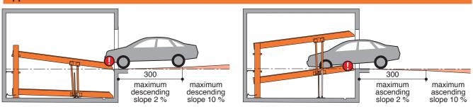
The illustrated maximum approach angles must not be exceeded. Incorrect approach angles will cause serious maneouvring & positioning problems on the parking system for which the local agency of KLAUS Multiparking accepts no responsibility.
