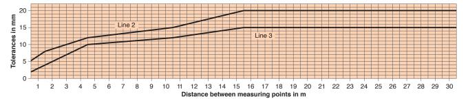
Intermediate values are to be taken out the diagram and must be rounded-off to mm.
