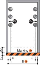
Units are dowelled to the floor. Drilling depth: approx. 15 cm.
