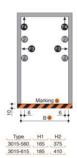
Units are dowelled to the floor. Drilling depth: approx. 15 cm.
