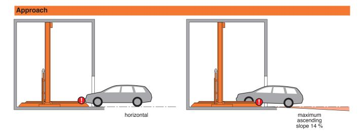
The illustrated maximum approach angles must not be exceeded. Incorrect approach angles will cause serious maneouvring & positioning problems on the parking system for which the local agency of KLAUS Multiparking accepts no responsibility.
